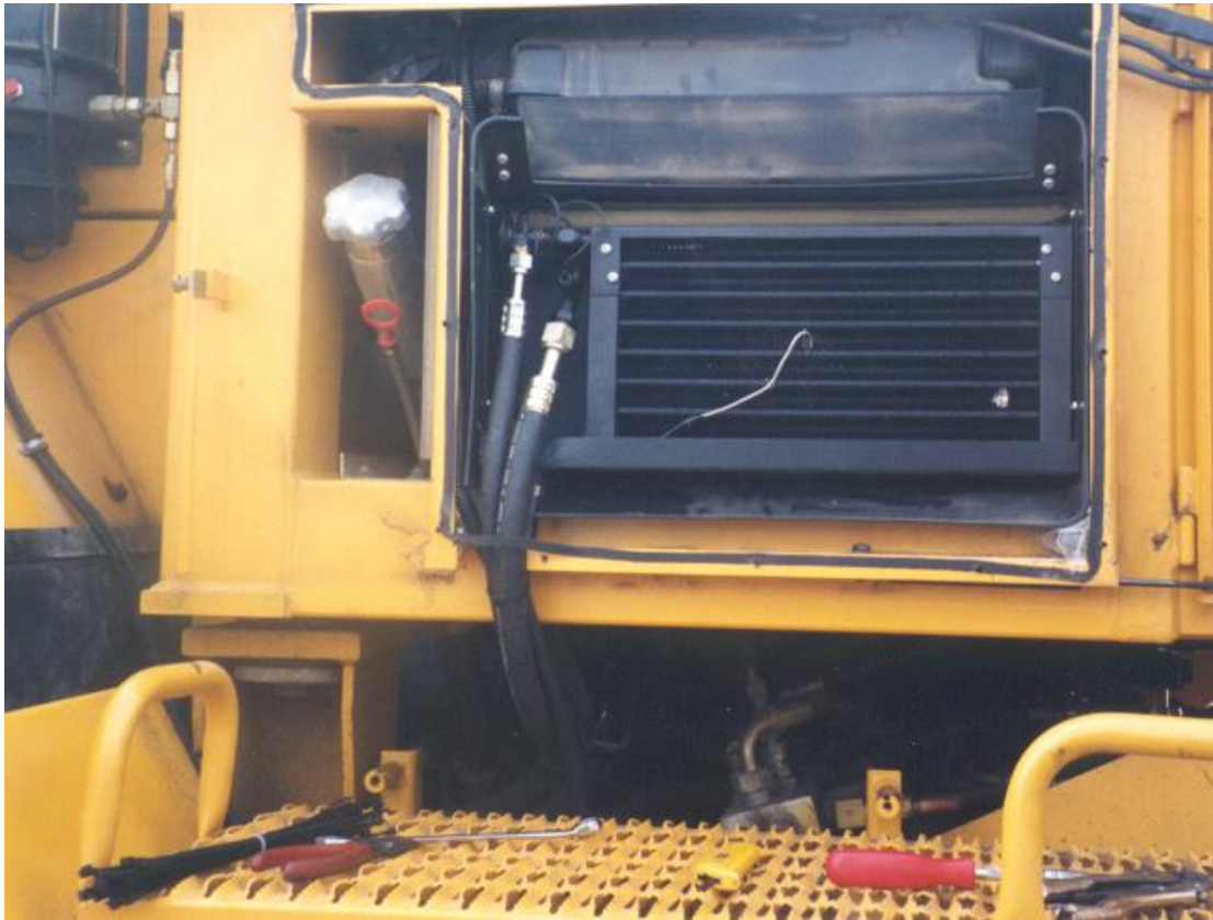
Face on view of evaporator with hoses and thermostat probe.
