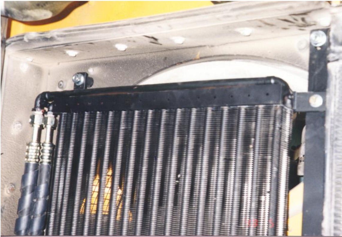
Condenser view showing upper mount points and fitting arrangement.
