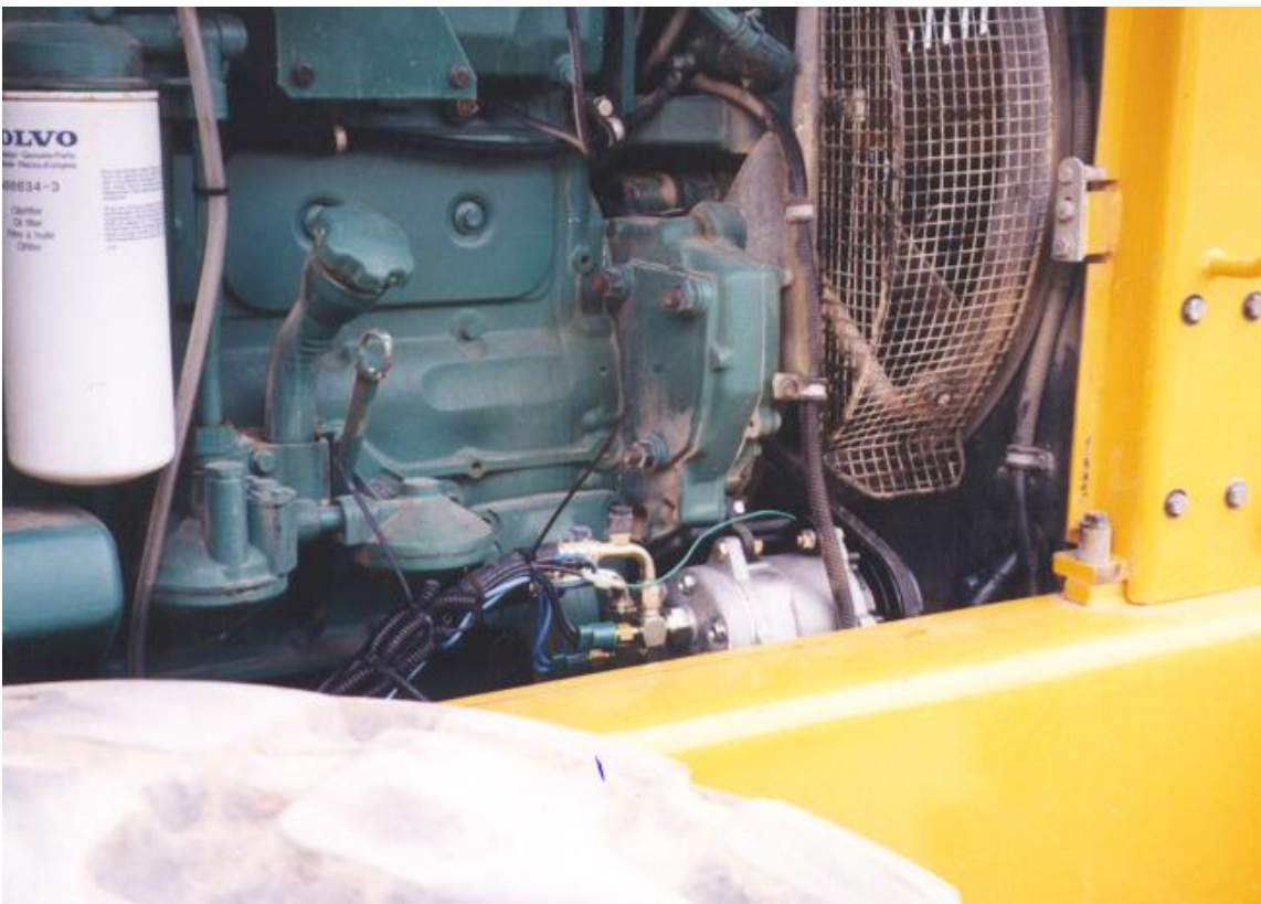
Compressor in place showing line runs.
