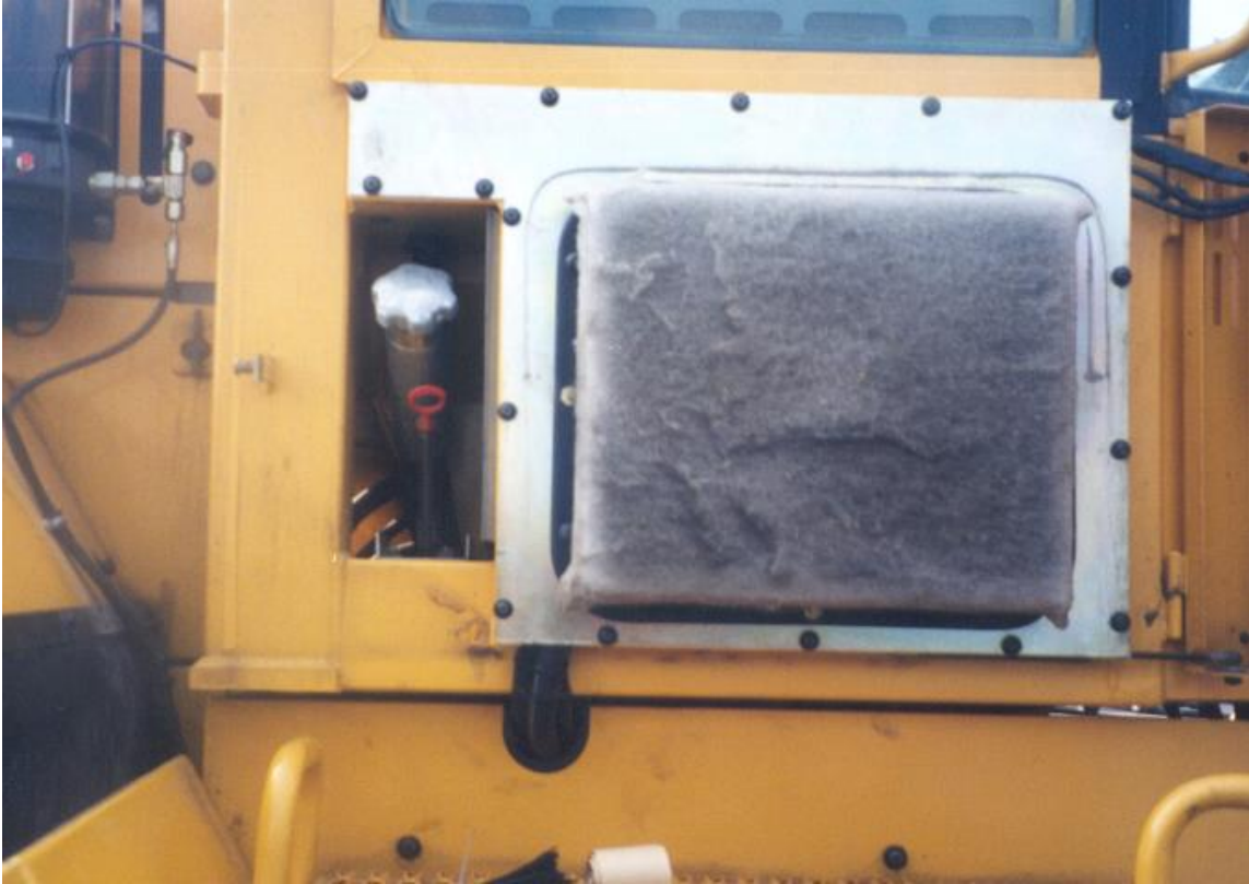
Filter assembly in position with pre-filter in place.
